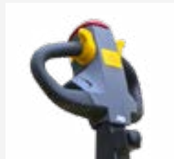
Adjustable, Ergonomic Tiller Head
