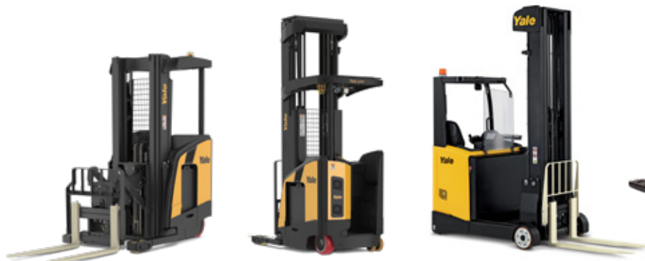
NR/NDR030-040DC ★ Pantograph 3,000-4,000 lbs. NR/NDR030-045EC ★★ Pantograph 3,000-4,500 lbs. MR14-25A (Indoor) ★ Moving mast 3,000-5,500 lbs.
