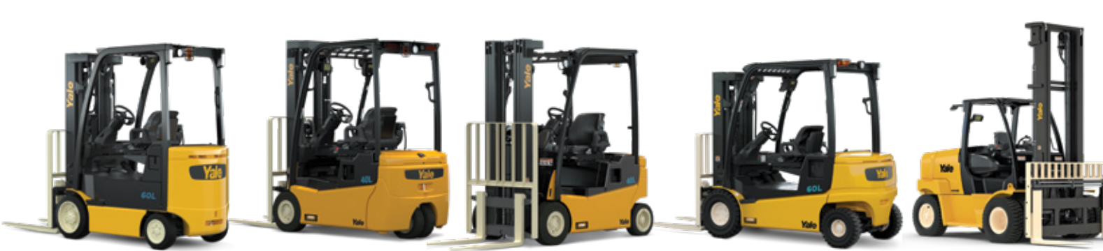
ERC050-060VGL ● Cushion tire 5,000-6,000 lbs. ERP040VTL ★★ 3-wheel pneumatic tire 4,000 lbs. ERP040VFL ● Pneumatic tire 4,000 lbs. ERP050-060VLL ● Pneumatic tire 5,000-6,000 lbs. ERP155-190VNL Pneumatic tire 15,500-19,000 lbs.
