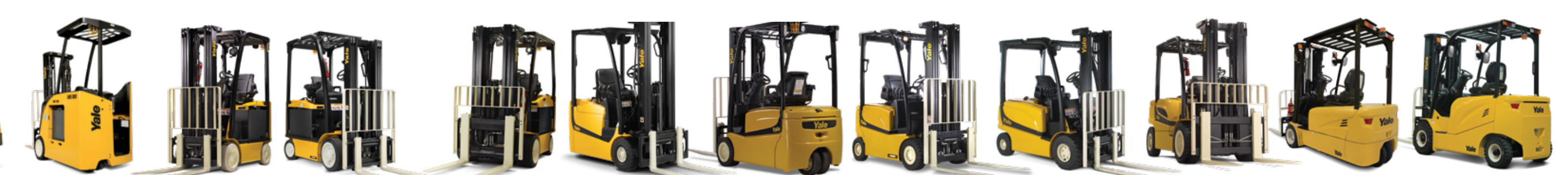
ESC030-040AD ★★ 3-wheel stand-up 3,000-4,000 lbs. ERC030-040VA ● Cushion tire 3,000-4,000 lbs. ERC045-070VG ● Cushion tire 4,500-7,000 lbs. ERC080-120VH ● Cushion tire 8,000-12,000 lbs. ERP025-030VC 3-wheel pneumatic tire (RWD) 2,500-3,000 lbs. ERP030-040VT ● 3-wheel pneumatic tire 3,000-4,000 lbs. ERP030-040VF ● Pneumatic tire 3,000-4,000 lbs. ERP045-070VL ● Pneumatic tire 4,500-7,000 lbs. ERP080-120VM ● Pneumatic tire 8,000-12,000 lbs. ERP32-40UXT 3-wheel pneumatic tire 3,200-4,000 lbs. ERP30-70UX Pneumatic tire 3,000-7,000 lbs.
