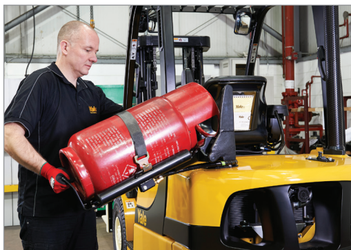
EZ™ – Swing out, drop down LPG bracket
