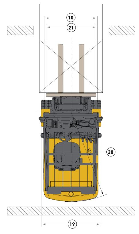
Yale uses the above ITA formula to calculate Right Angle Stack on our 3 and 4 wheel trucks with a zero turn steer axle and counter rotating load wheels.
