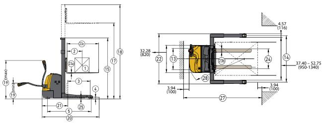
$Circled\ truck\ dimensions\ correspond\ to\ the\ line\ numbers\ in\ the\ General\ Specifications\ chart.\ Dimensions\ are\ listed\ in\ inches\ (millimeters.)$
