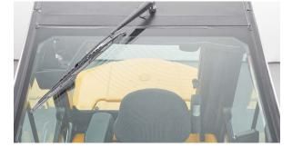
A laminated glass top canopy option provides an unobstructed upward view to support precision and productivity while picking and placing loads at height.
