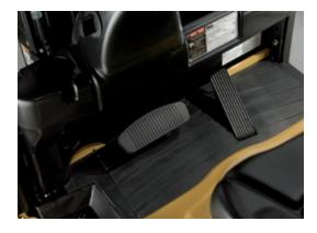
**ELECTRIC PARKING BRAKE** Engages when truck stops, simplifying operation.
