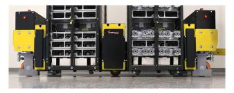
Powered by the automated tugger, the dual bay server racks can lift and lower ORV2/ORV3 data servers for transport.
